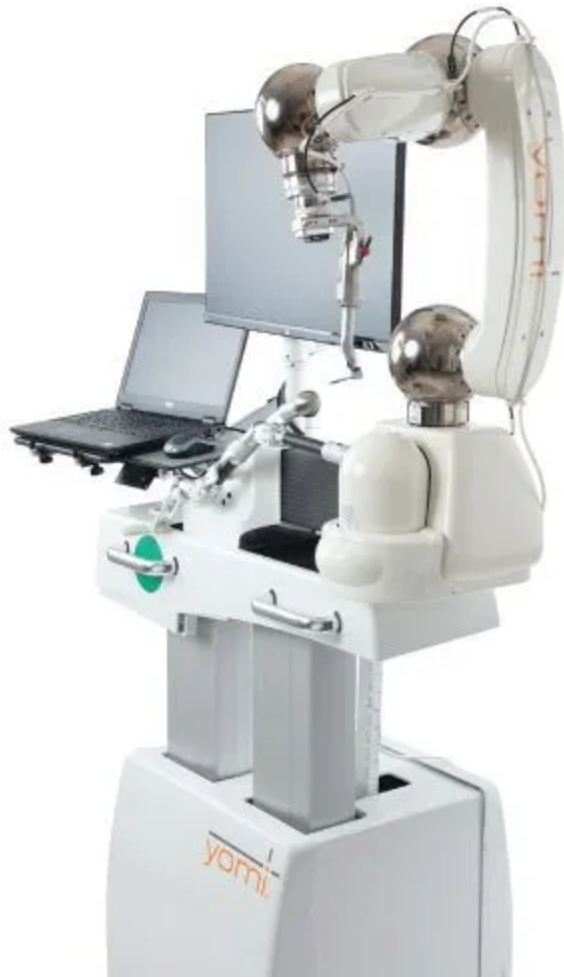
Figure 1. The Yomi robotic system (Neocis Inc). »
